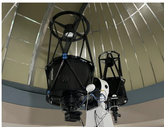
Fig. 1. The PNUO telescope system. The 0.5m telescope is co-mounted on the same mount with a 0.36m telescope for visual observation.
